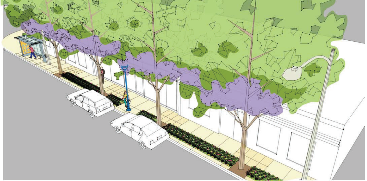
Aerial view of City improvements where existing sidewalks are 9' 6" wide.
