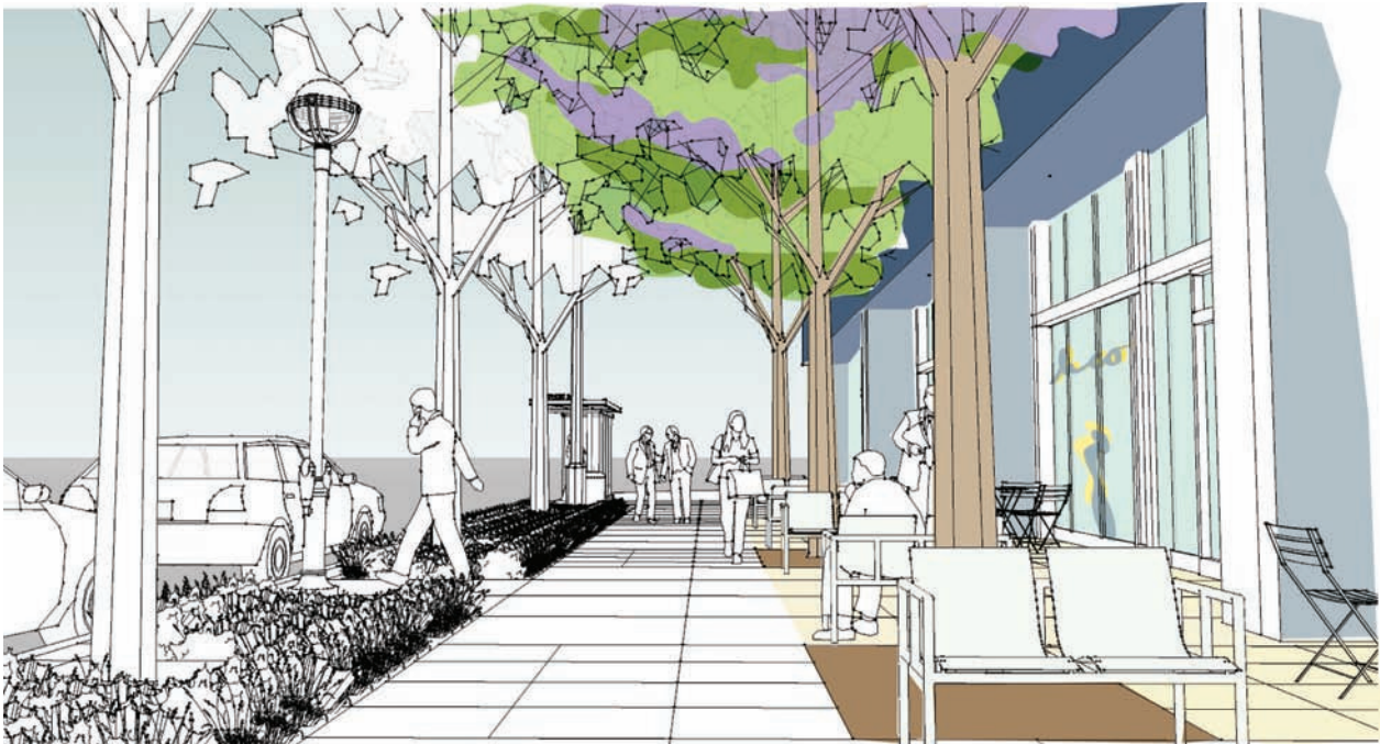
Sidewalk view of future improvements where existing sidewalks are 25' wide, similar to the western portion of Santa Monica Boulevard. One of the defining elements on Santa Monica Boulevard is the double row of trees in locations where the sidewalk is at least 24' wide. While 25' wide sidewalks are not required on La Brea Avenue, developers are encouraged to incorporate them along some of their street frontage to provide opportunities for outdoor dining and additional landscaping, including a second row of trees which may be either aligned with the street tree, as on Santa Monica Boulevard, or staggered.
