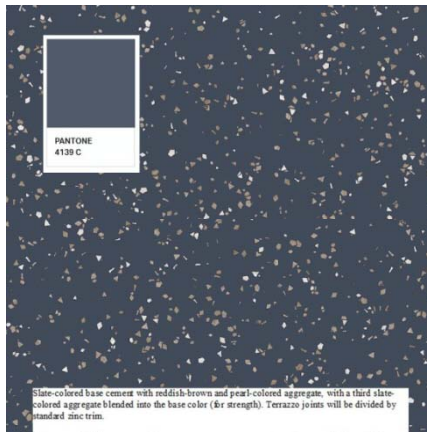
'Primary' Terrazzo Slate-Colored base 'Pantone' w/ selected exposed aggregate. Rated for outdoor use.
