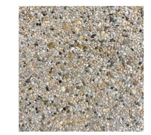
Special Casting Finish 'Primary' Decorative Concrete with an Integral warm gray color to be selected. The finish will be a Special Casting which is seeded over the top and troweled in, with saw cut score lines. See plan for scoring pattern
