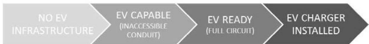
Figure 1: Four Levels of EV Charging Readiness
